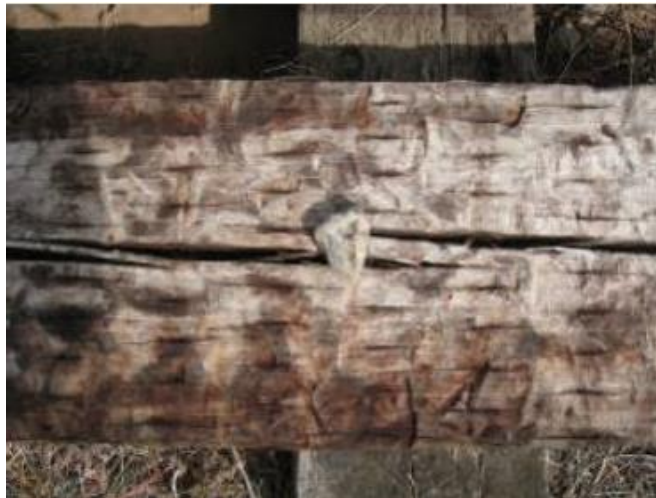
Figure 2.3 Underside of a conventional wood tie removed from service showing indentations from ballast particles. (FRA Task Order 225)
