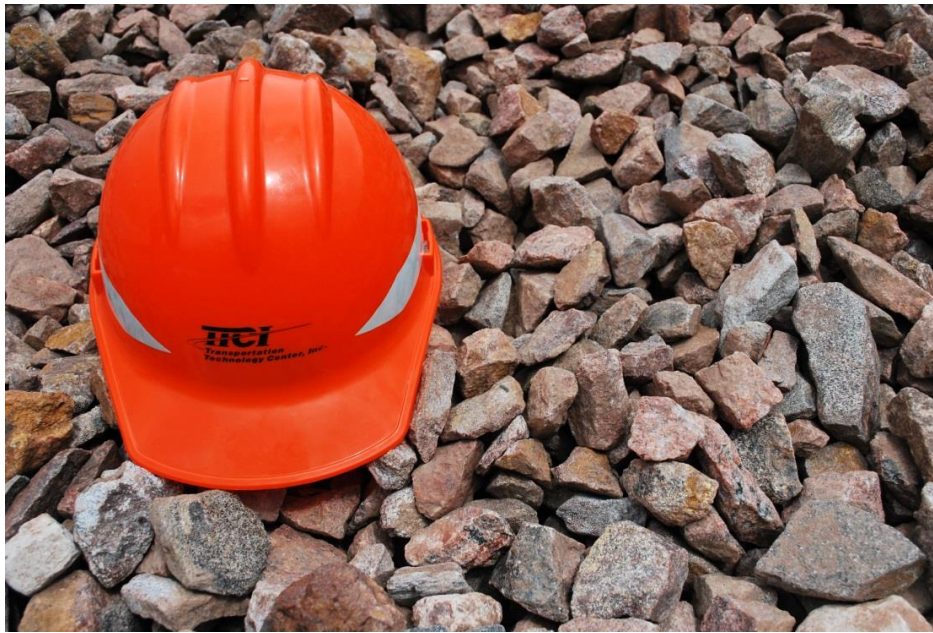
Figure 1.2 Example of new, conventional, mainline, crushed rock ballast
